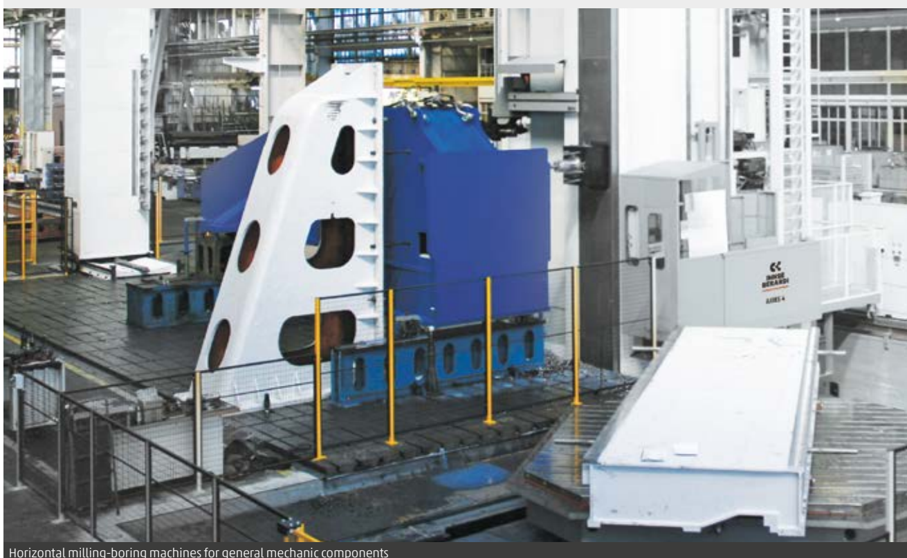
Horizontal milling-boring machines for general mechanic components
