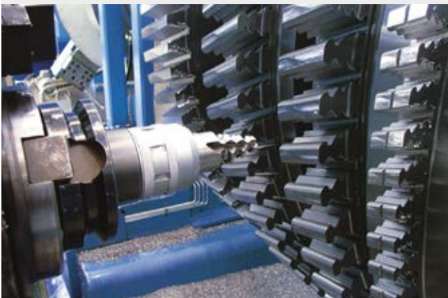
Rotor slotter for turbine rotors
