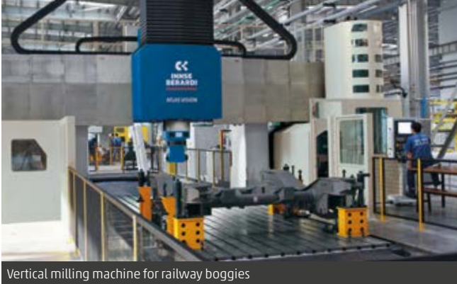
Vertical milling machine for railway engines
