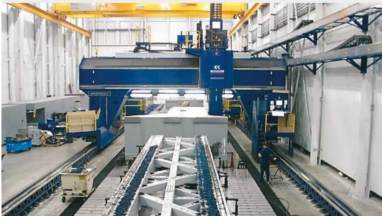
Horizontal milling-boring machines for general mechanic components
